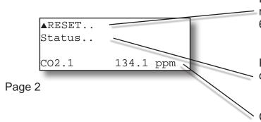
Press the ← key in this line to enter a submenu to reset the calibration parameters (■ 6.2.2.2.1, page 6-8)
